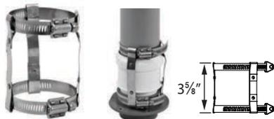
Use to secure PolyPro pipe to PVC/CPVC coupler or appliance outlet. Universal size for 2-4 inch and 5-8 inch systems. DuraVent requires its use with flue gas applications and recommends it with air intake applications.
