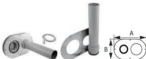
Use to adapt PolyPro to the IpeX 636 low profile termination. Kit includes 14" pipe welded to an adapter and metal backing plate. Check with appliance manufacturer for approval. (Outer IPEX termination cap not included. Supplied by others.) Includes 1 Locking Band.
