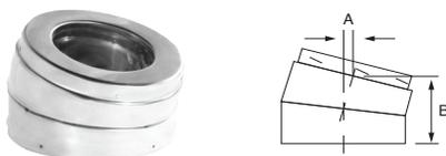
Allows the 15° offset of a chimney. Designed to bypass an obstacle, such as a joist. A maximum of two offsets (4 elbows) is allowed.
